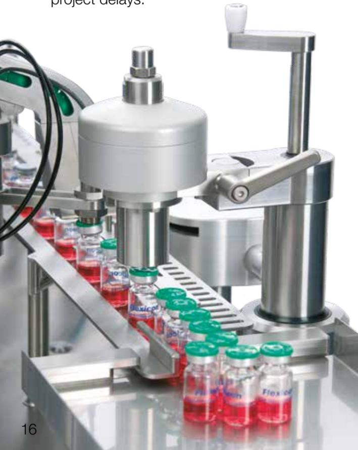
FPC50 crimping head for minimum air turbulence and fast changeover between caps
