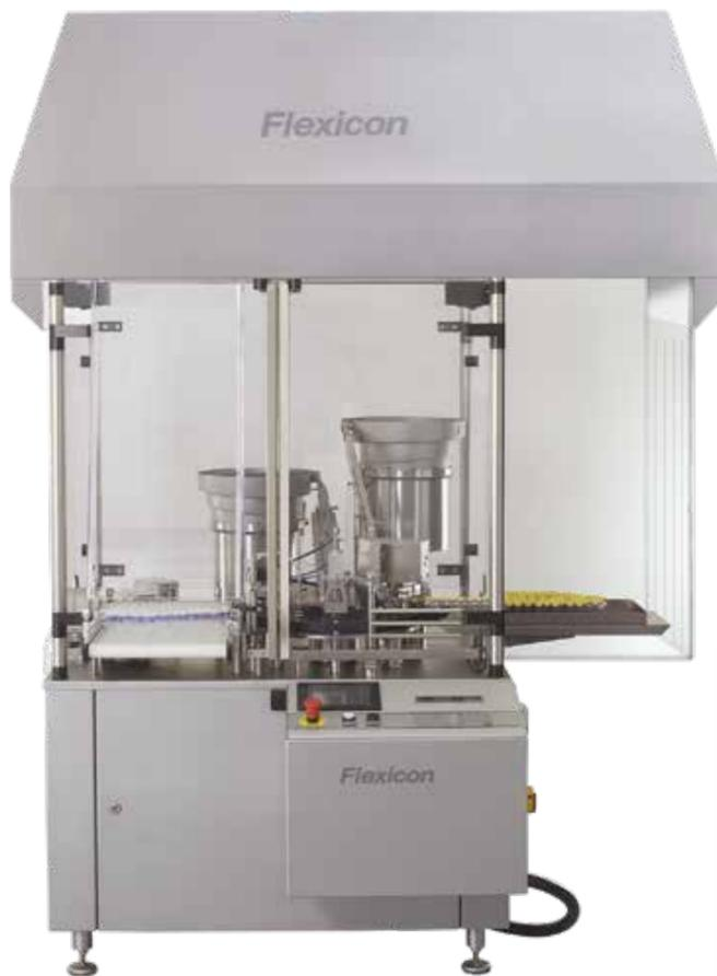
Above: An FMB210 installed within a laminar air flow cabinet.
