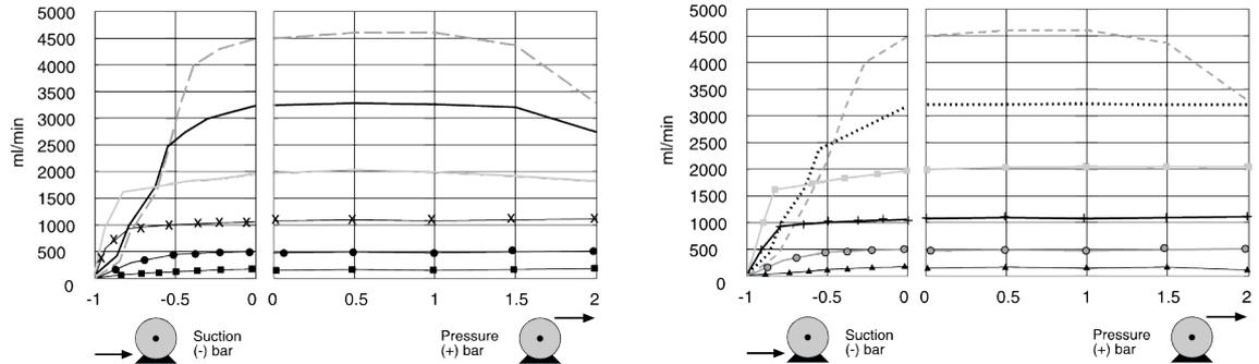
521R2C Pumphead performance curve, with Marprene tubing at 291rpm
