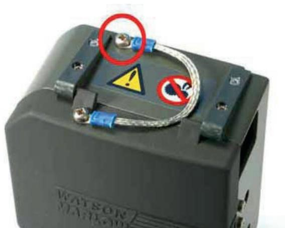
It is possible to check the effectiveness of any earth connection by measuring its electrical resistance. The resistance from any point on the safeguard to the earth terminal is typically 25 Ohms. **To ensure reliable dissipation of static the maximum resistance to earth should not exceed 1 MOhm.**
