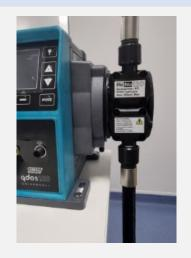
The pump must be located upon a plinth with a minimum height of 180 mm (7.09") to the bottom of the pumphead fluid connection
