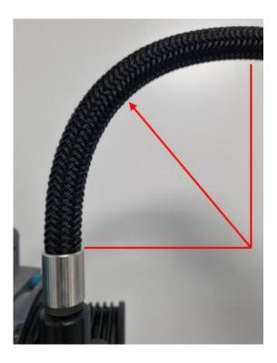
In order to avoid bending the hose below the minimum bend radius, it may be necessary to uninstall and re-mount a qdos pump, prior to installing a qdos hose connector kit.
